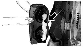
4. Remove the three screws holding the bulb strip to the back of the tail lamp.
